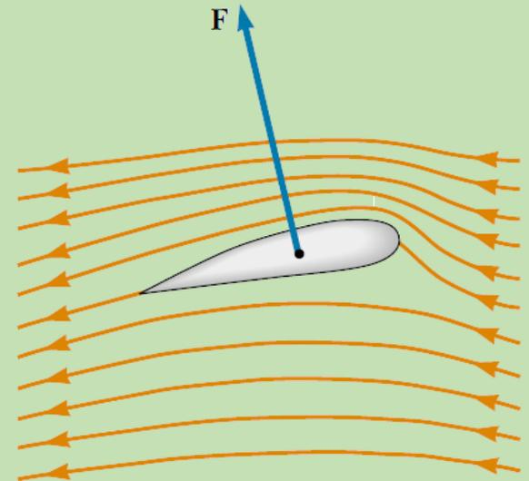
$$F = PA = (P_{\text{sup}} - P_{\text{inf}}) A = \Delta PA = 1.42 \times 10^6 \text{ N}$$
